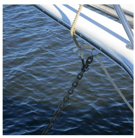
Mark is in the process of putting on a snubber in this photo.
