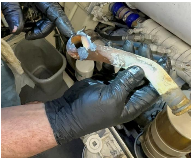
This is the broken pipe.
