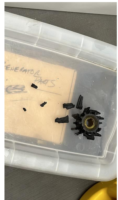
The broken impellor.
